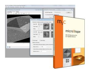
M2C microShape software creates, visualizes and analyses 3D surface models from SEM images. Your SEM must be equipped with a 4-quadrant backscatter electron (4Q BSE) detector. Generating 3D data is quick and simple: it only takes a few seconds to create and visualize the topography of your samples.
