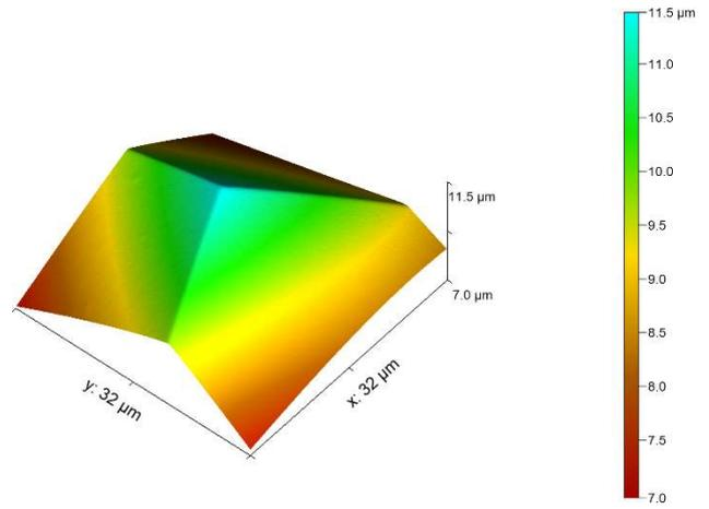
Fig. 2: 3D Reconstruction of a Berkovich indenter tip.
