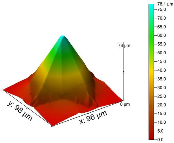
Fig. 1: 3D Reconstruction of a silicon microprobe tip.
