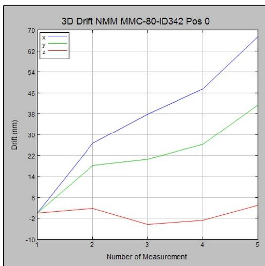
Figure 2: Lateral and vertical drift for repeated measurements by the Met. LR-AFM over 16.8 hours
