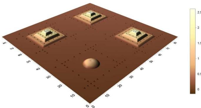
Figure 1: 3D calibration standard, 3D view of AFM measurement data (units in  $\mu\text{m}$ )
