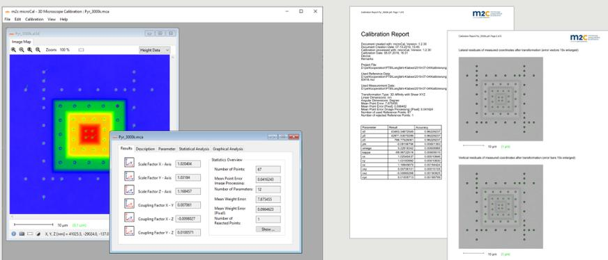
Figure 2: 3D calibration software "microCal" with 3D SEM data (left), first two pages of the automatically generated calibration report (right)
