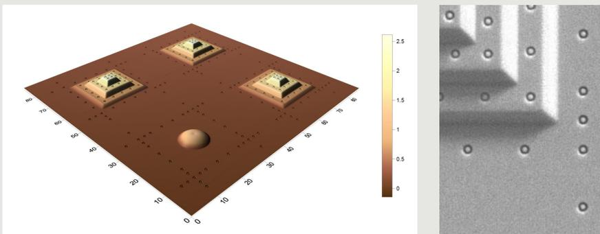
Figure 1: 3D calibration standard with reference marks, 3D view of AFM measurement data (left, units in  $\mu\text{m}$ ), Detail (right, SEM image)
