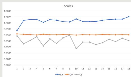
Figure 4: 3D calibration of the applied CLSM with a 3D calibration standard traceable to Met. LR-AFM during a period over 1.5 years (02/2018-08/2019). X-axis represents the series of measurements in the mentioned period, which is not equivalent to the time axis.
