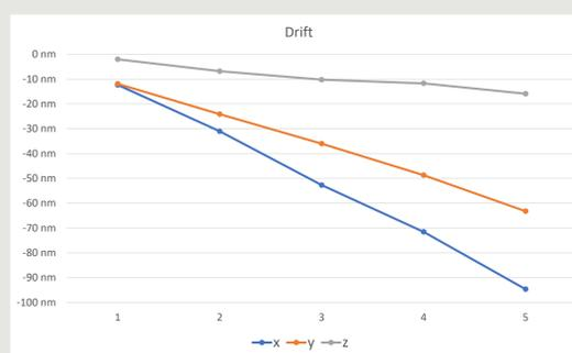
Figure 3: Typical drift of the applied CLSM (08/2019). X-axis shows the number of the measurement, which is not exactly the time axis.
