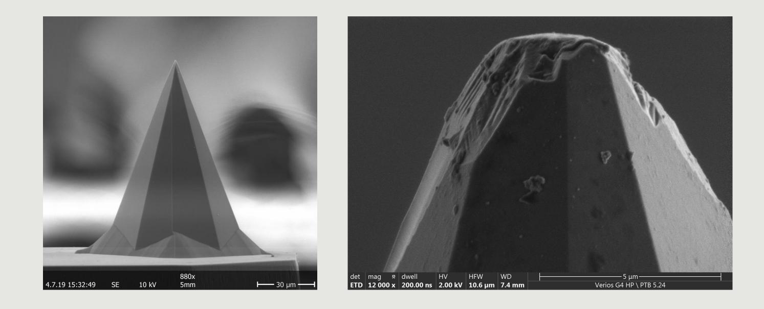
Figure 1: Si-tip (left, side view), wear effects on top of a Si-tip (right)
