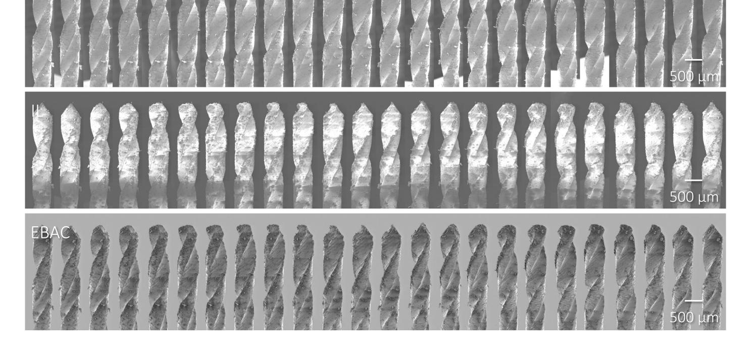
A standard 0.5 mm drill piece was placed in an electrical holder on the SEM stage, standing normal to the stage. The stage was tilted to 75° and rotated by 15° for a series of 24 micrographs covering the entire 360° range.
