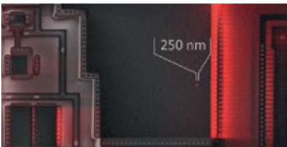
Colour mix of black-white SE and black-red RCI signals showing a CMOS capacitor with a leakage failure point (plan view, 38.5 μm image width)
