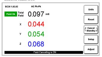
Fig. 1. Typical touch screen display
