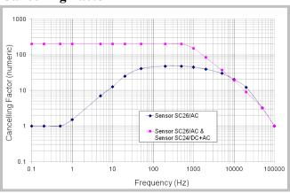
The "cancelling factor" is the ratio of the ambient field to the cancelled field. A graph of cancelling factor vs. frequency is above.
