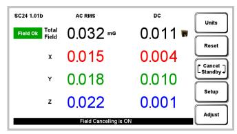
Fig. 2. Typical touch screen display with DC sensors
