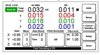
"Setup" automatically sets the feedback loop gains and phases. The gain values are displayed for reference. There is no manual adjustment.
