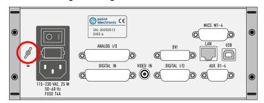
Connect the device to the supply voltage.
