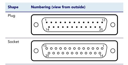
**Assignment** The following table contains information on the assignment of the connection numbers:
