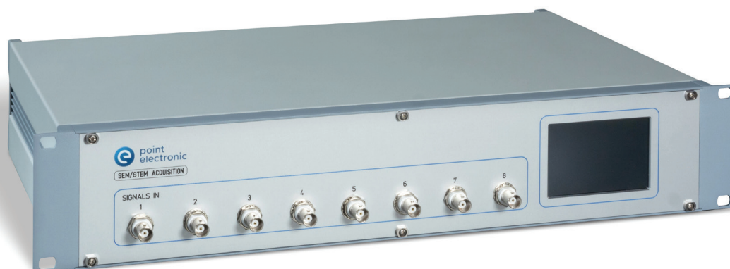
FIGURE 1 Photo of DISS6 scan generator hardware. To assist software development, display on front panel shows parameters of running scan job.
