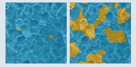
Classification results as coloured overlay with SE image (blue: grain boundaries, yellow: cleavage areas). Left: Predicted surface characteristics from SE images only, right: improved results with additional topographic data
