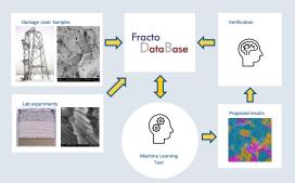
Principle of software assisted fractography: Application of machine learning tool and knowledge base. Verified results improve the data base.
